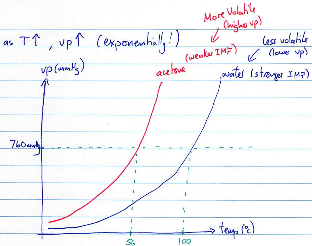
When  $vp = \text{external/atmospheric pressure}$ , we get BOILING!
